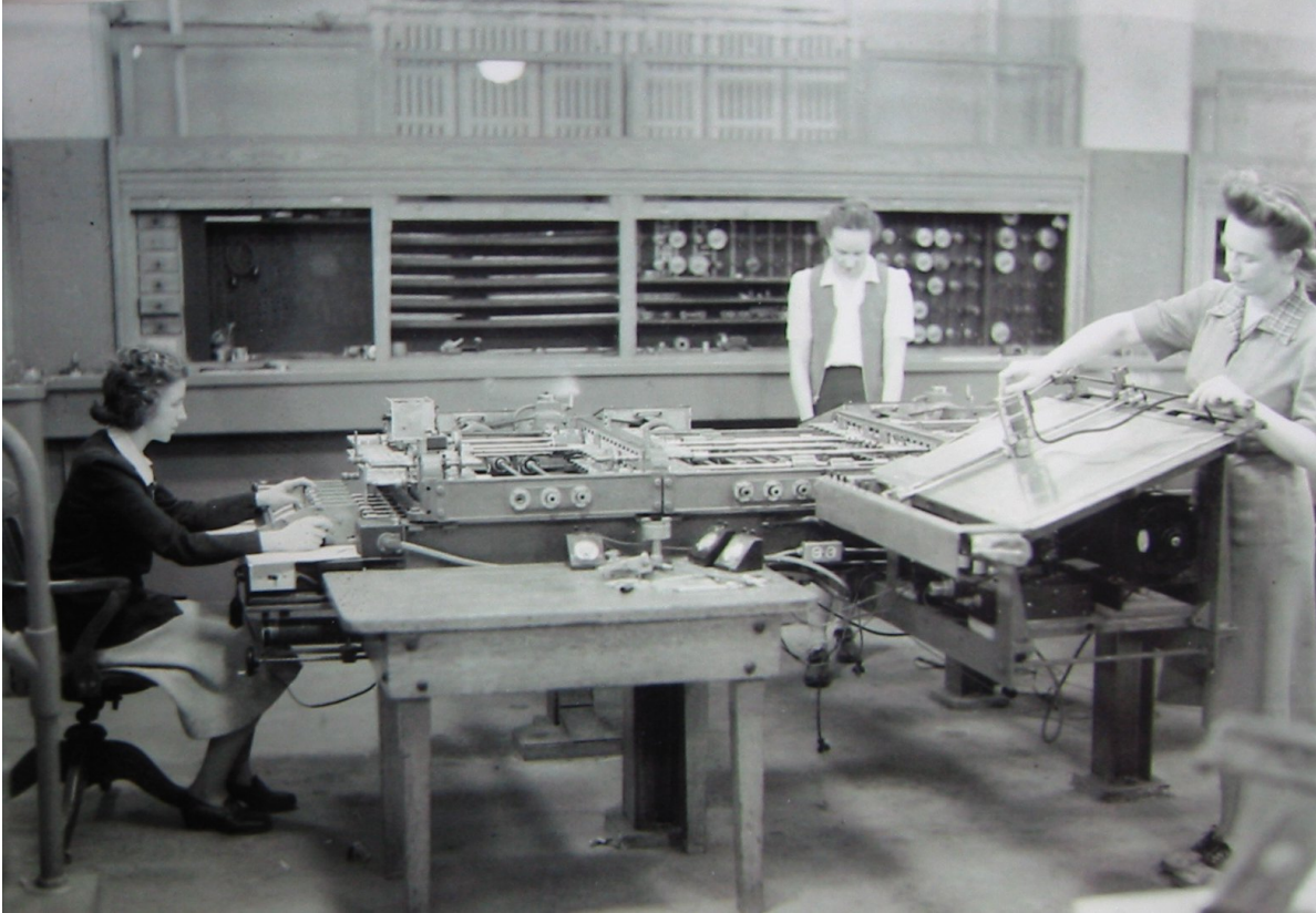
Figure 1: Kay McNulty, Alyse Snyder, and Sis Stump operate the differential analyser at the Moore School of Electrical Engineering, University of Pennsylvania, c. 1942–45. US Army photograph; public domain via Wikimedia Commons .
